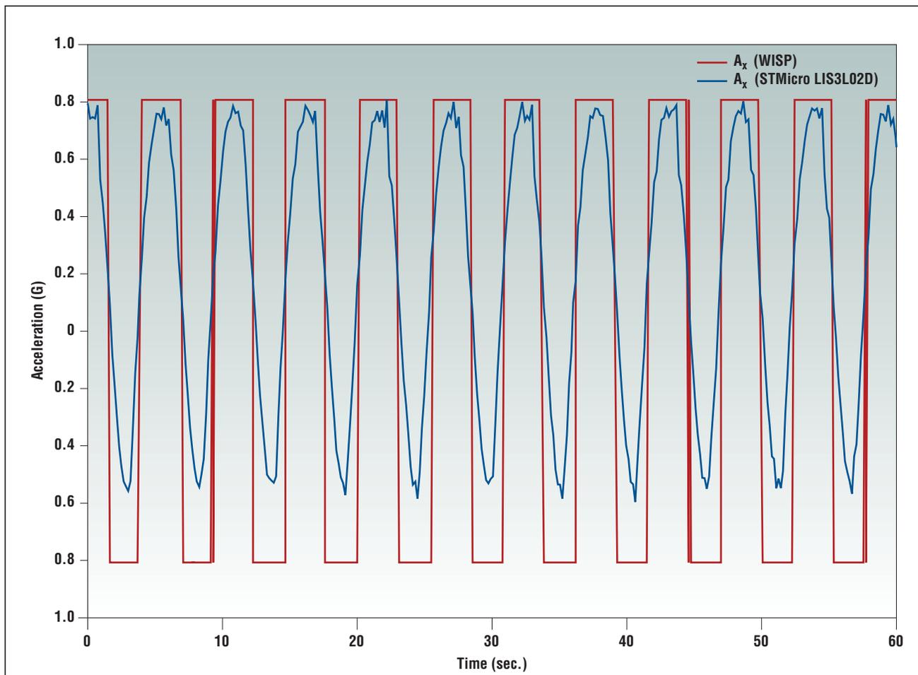
Figure 4. An  $\alpha$ -Wisp parasitically powered one-bit accelerometer in operation. Comparison of data returned by the  $\alpha$ -wisp (the red trace) with continuous acceleration data provided by an STMicroelectronics LIS3L02D three-axis accelerometer (the blue trace).
