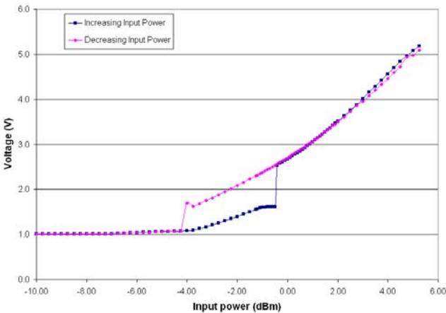
Fig. 5 Rectified voltage vs. input power measurements using a network analyzer for RF signal insertion in to the antenna ports.
