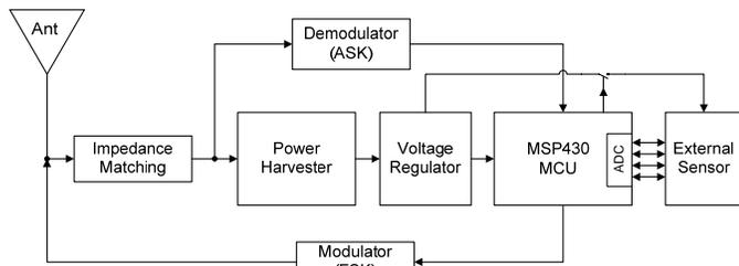
Fig. 2 Block Diagram of the WISP platform
