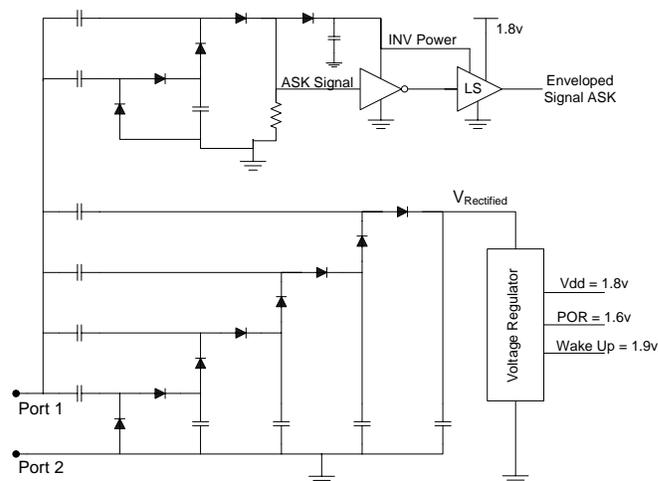
Fig. 3 Schematic of WISP power harvesting and communication circuit.
