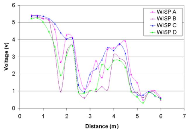
Fig. 6 Rectified voltage in sleep mode vs. distance for an RFID reader
