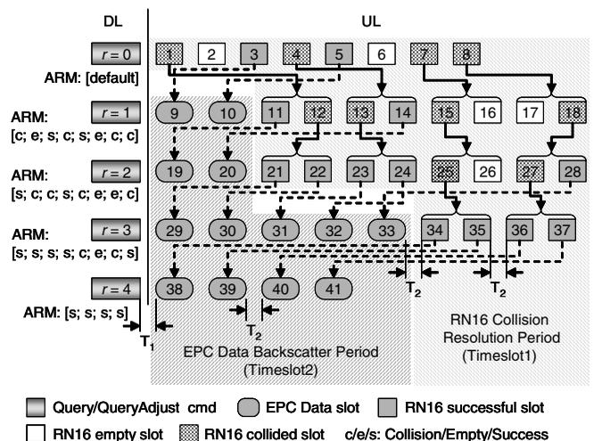
Fig. 2. Collision resolution process in BMSA ( $m = 2$ )
