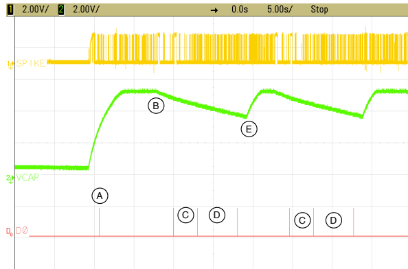
Fig. 9. Two read cycles of wireless operation, showing the spike detector output (top), the unregulated stored voltage (middle), and a microcontroller output (bottom) pulsed to show operation. The data was taken at a distance of approximately 1m from the reader.
