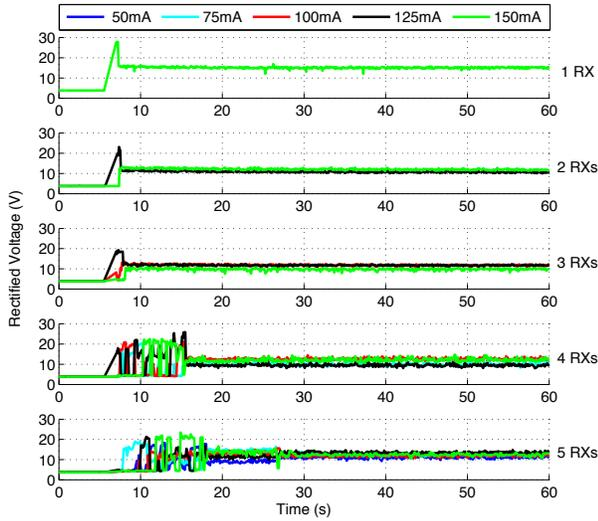
Fig. 5. Rectified voltage for 1-5 receivers using adaptive tuning techniques.
