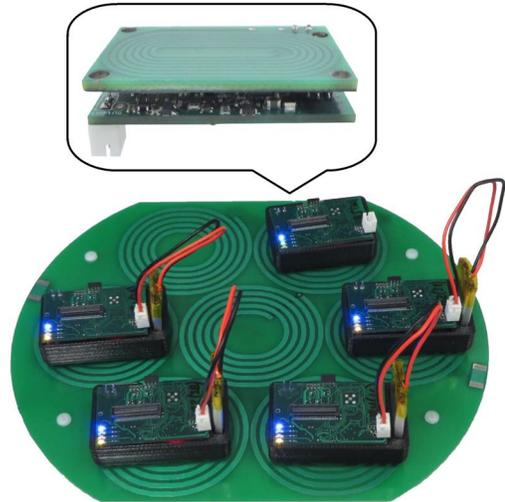
Fig. 3. Transmit coil array powering five receivers simultaneously
