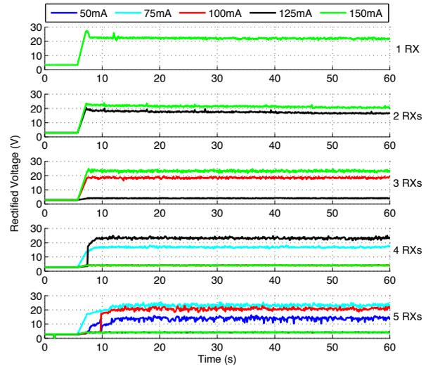
Fig. 6. Rectified voltage for 1-5 receivers without adaptive tuning.
