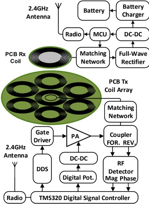
Fig. 1. Schematic diagram of the proposed wireless power system.
