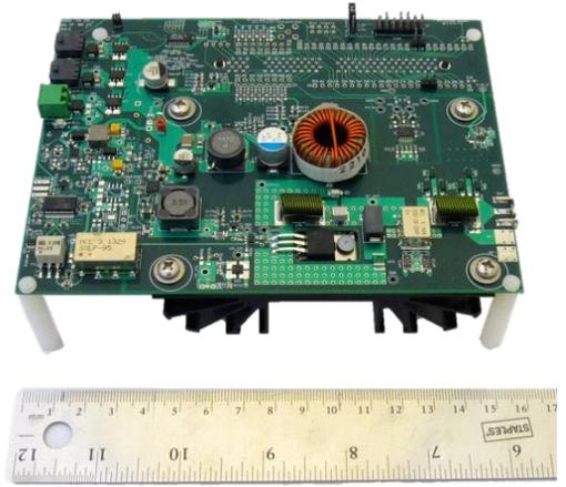
Fig. 2. Transmit controller and power amplifier PCB.
