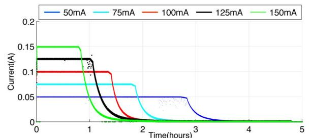
Fig. 4. Charge current for five wirelessly powered battery chargers.
