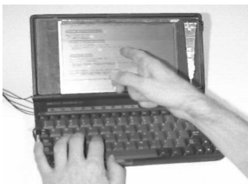
Figure 7. Two-dimensional finger-pointing mouse. 2-D Finger-Pointing Mouse
