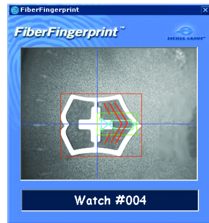
Figure 1. FiberFingerprint scan of watch logo. Unique surface irregularities can function as an identifier in physical objects to prevent forgery and product diversion. Image courtesy of Escher Group, Ltd.
