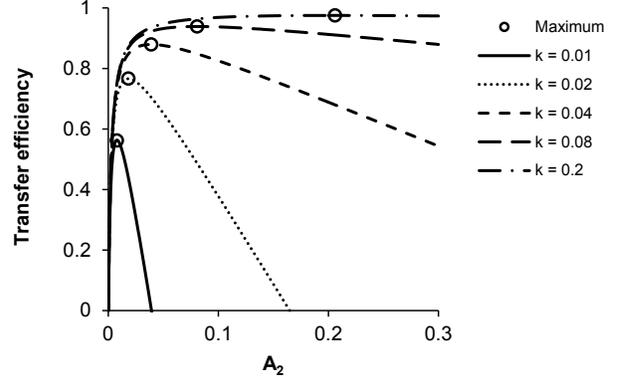
Fig. 3. Transfer efficiency vs.  $A_2$  in the range of  $k_{critical}$ .  $Q_2 = 418.6$ ;  $Q_3 = 384.6$ .
