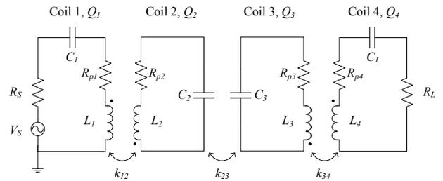
Fig. 1. Equivalent circuit model of a 4-element WPT system showing the source voltage ( $V_s$ ), source resistance ( $R_s$ ), load resistance ( $R_L$ ), parasitic resistance ( $R_{pn}$ ), inductance ( $L_{pn}$ ), capacitance ( $C_{pn}$ ) and quality factor ( $Q_n$ ) of the  $n^{th}$  coil.
