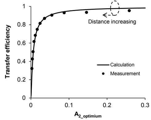
Fig. 5. Comparison result of transfer efficiency between calculation and measurement in function of  $A_{2\_optimum}$  in the range of distance.
