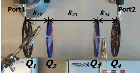
Fig. 4. Photograph of the 4-element WPT system.  $Q_{1,4} = 1.9$ ;  $Q_2 = 418.6$ ;  $Q_3 = 384.6$ . The copper wire (1.024-mm thickness) is used for coils.
