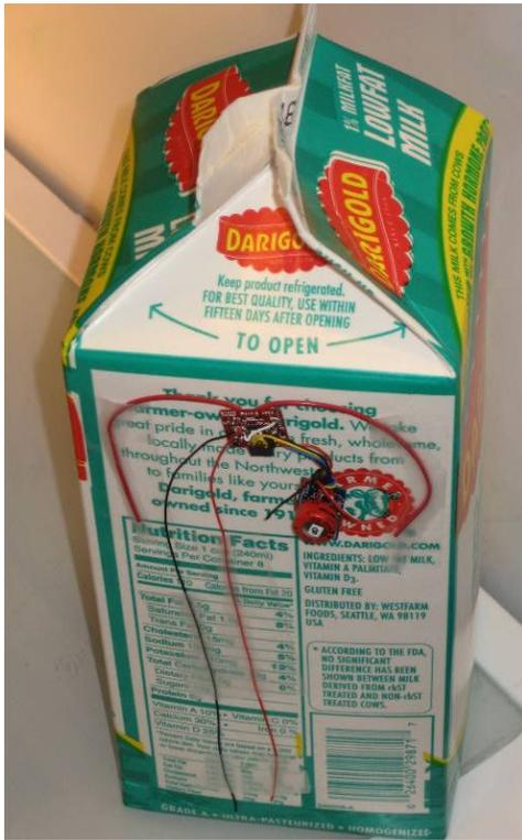
Figure 2—Picture of WISP and fill sensor on milk carton
