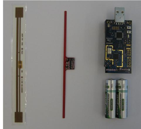
**Figure 1**—A standard UHF Class 1 Gen 2 RFID tag, Intel WISP, and Telos Mote (left to right)
