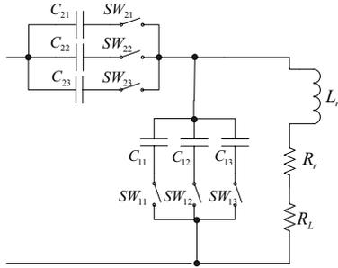
Fig. 7. The schematics of the adaptive L-match network.
