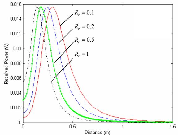
Fig. 6. The demonstrated relationship between the received power and coupling factor, which is simulated with a reader antenna with  $S=20\text{cm} \times 20\text{cm}$  and one turn, a tag with  $S=0.023\text{m}^2$  (10 turns) and  $R_t=6.2 \Omega$ ,  $V_p=5$ , and  $R_{sr}=50 \Omega$ .
