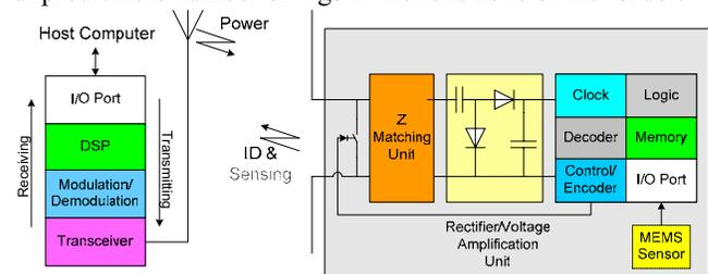
Fig. 1. The RFID reader-tag (sensing node) system
