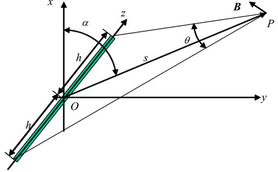
Fig. 3. Magnetic field generated by a dipole.
